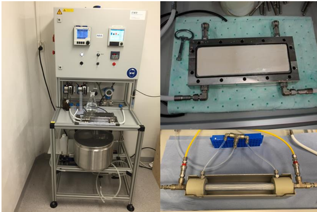
Figure 2. Membrane filtration unit (left) and membrane test cells used for nanofiltration investigations at NIVA at a bench scale: right top: cell for flat membranes, right bottom: cell for hollow fibre membranes (Photos: P. Krzeminski).
