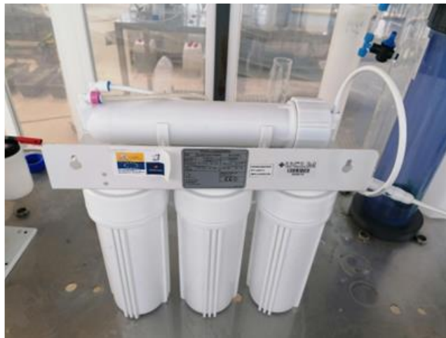
Figure 3. Commercial reverse osmosis equipment investigated at UCLM (Spain) as an alternative to nanofiltration unit.
